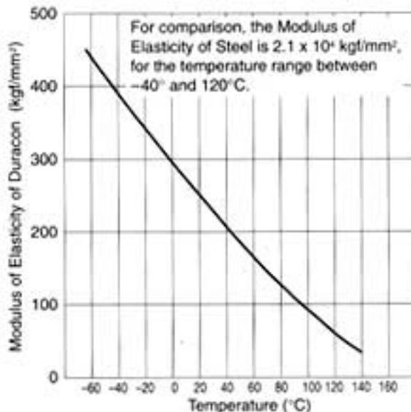
**Fig. 18-5 Modulus of Elasticity in Bending of Duracon**
