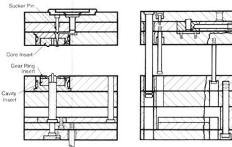
(b) Gates Separated from Molded Parts
