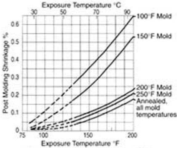
Fig. 18-7 Shrinkage for Delrin in Air
