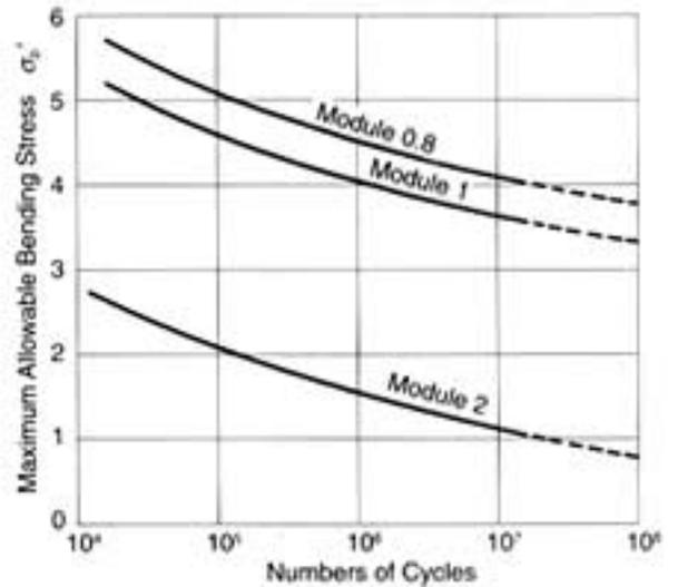
Fig. 18-2 Maximum Allowable Bending Stress under Ideal Condition,  $\sigma_b'$  (kgf/mm<sup>2</sup>)
