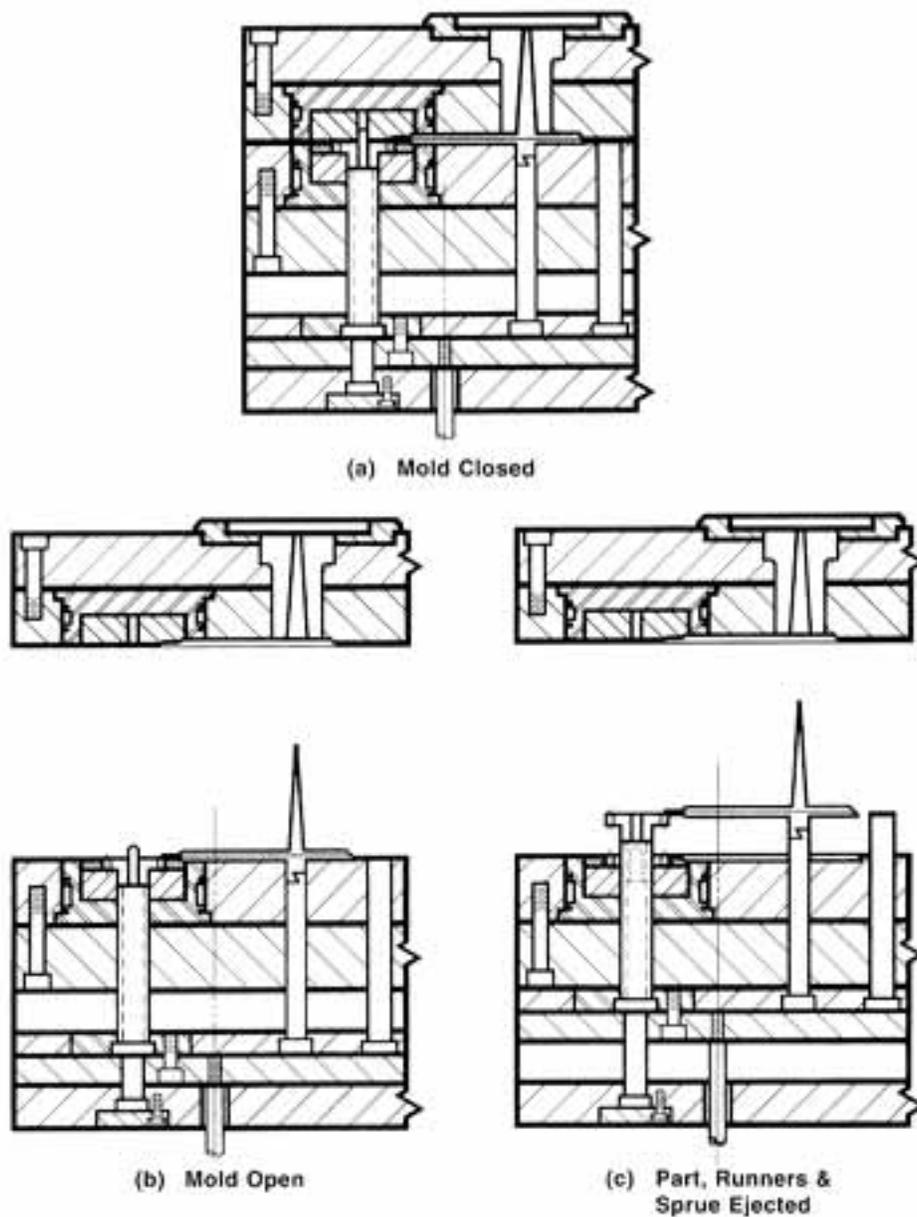
Fig. 18-15 Two-Plate Mold
