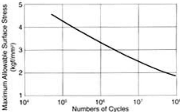
**Fig. 18-6 Maximum Allowable Surface Stress (Spur Gears)**
