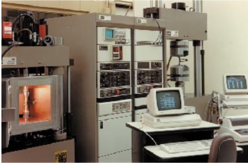
PLATE 15 Closed-loop, electro-hydraulic mechanical testing systems. (Photo courtesy MTS Systems Corp., Minneapolis, MN.)
